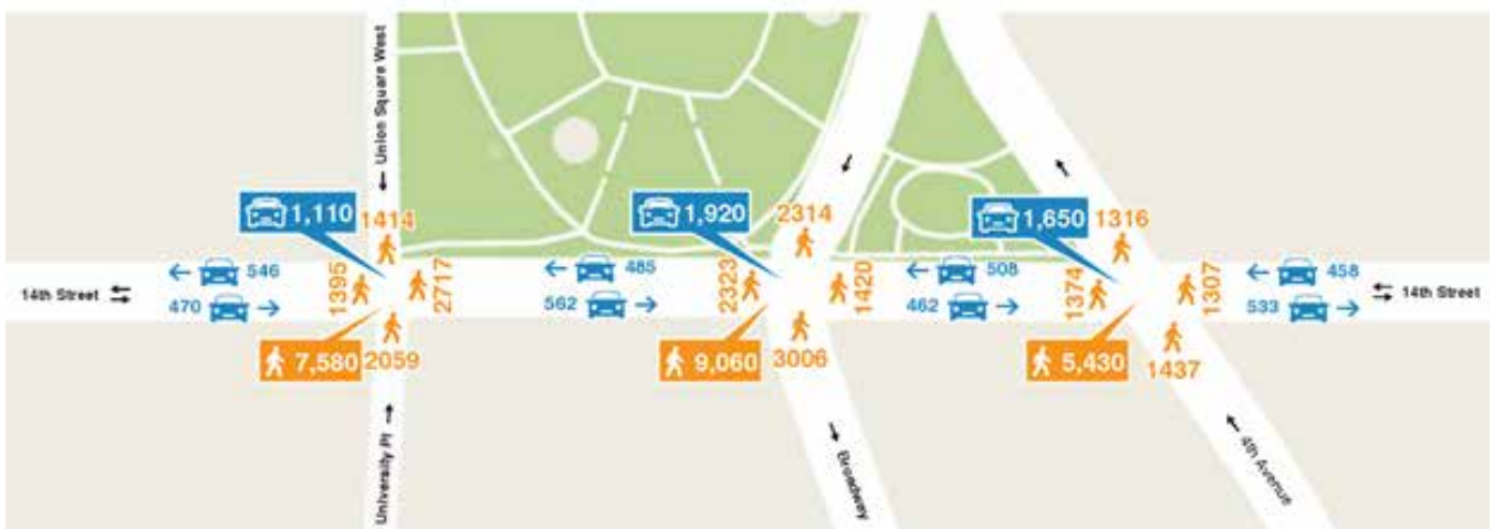
Diagrams illustrating pedestrian and vehicle volumes on the Union Square South section of 14th Street, between University Place and 4th Avenue.
